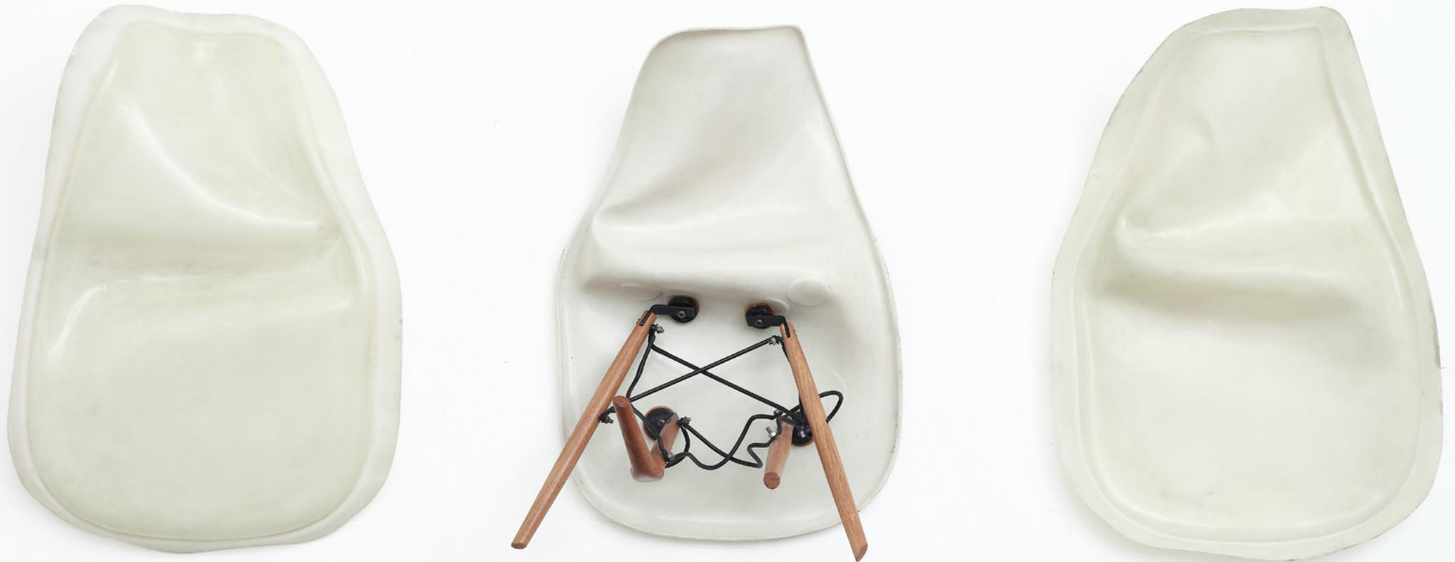
These are the mold parts for the front and back of the transformed seat shell, which was vacuum pressed to receive the same glass fibre structure as the original. For this shape a mold was created, based on a silicone casting produced using the original seat shell.
